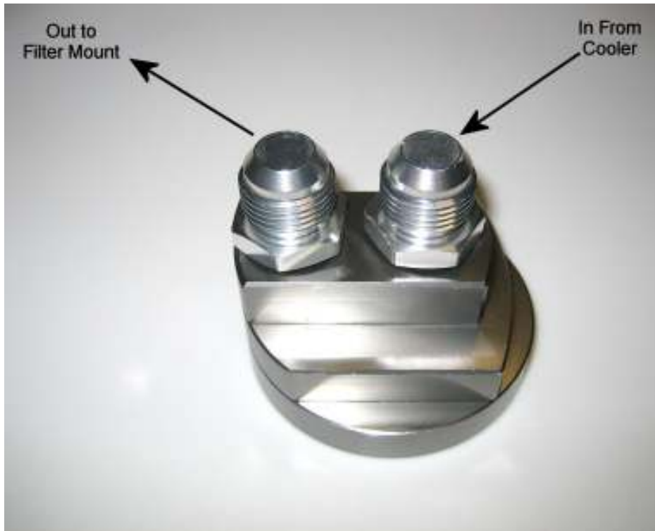
Figure 4: Block Adapter Oil Flow
